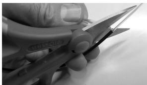
Check the correct insert or adjust the Mid-span access tool. The fibres should not be touched or damaged.
