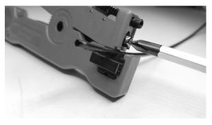
Adjust the Cable slit and ring tool. The tube should be cut without affecting the fibres.
