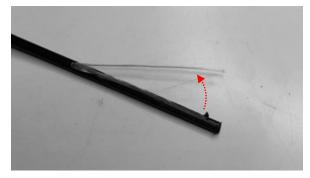
Pull the ripcord trough the outer sheath.
