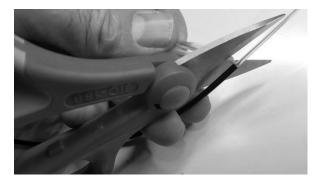
Cut the tube to a max length of 1cm from outer sheath using the Cable slit and ring tool.
