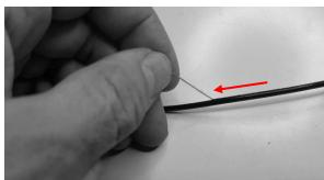
Cut the outer sheath and Aramid yarns using scissors.
