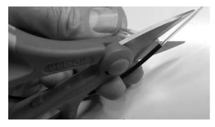
Cut the tube to a max length of 1cm from outer sheath using the Cable slit and ring tool.
