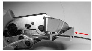
Cut the tube to a max length of 1cm from outer sheath.
